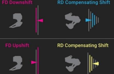
Compensating Shift smooths gear transitions. When a front gear change is performed, the rear derailleur compensates for the large change in gear ratio by shifting 1 or 2 cogs.
