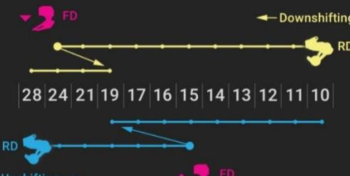
Sequential Shifting activates the next available gear using the left and right shifter buttons. Automatic actuation of the front and rear derailleurs keeps your gear ratio and pedaling cadence steady.
